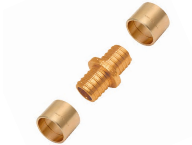
Fig. 49. KAN-therm Push connector for PE-Xc and PE-RT pipes, diameters 12 × 2, 14 × 2, 18 × 2, 18 × 2,5, 25 × 3,5
