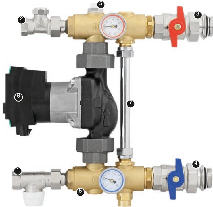
Mixing system is composed of a pump (three-stage or stepless depending on a version), ZR control valve, regulated by-pass, ZT thermostatic valve, 1" terminals to manifold and high-temperature installation, as well as 2 thermostats.
