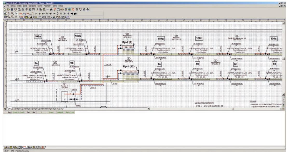
KAN C.O. Graf enables projecting the results of calculations onto floor plans (Fig. 81). To do this, draw a floor plan and then project heaters, pipes and other system components onto the plan. For simple shapes the software will draw underfloor heating coils. Once the calculations are complete, the software will describe the size of the heater and draw them to scale, it will provide pipe diameters and valve settings.
