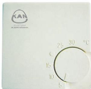
Basic bimetallic room thermostat is responsible for controlling executive elements - electric actuators in KAN-therm surface heating and allows for individual adjustment of temperature in room. The thermostat can be mounted inside flush-mounted box or directly on a wall. The device can operate in both 24V and 230V installation.
