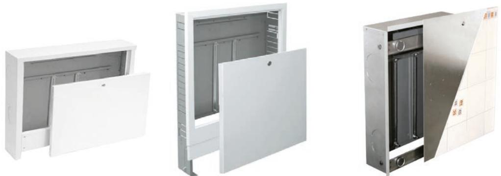
Flush mounted cabinets feature adjustable dimensions: height and width (SWP-OP) as well as depth (SWPG-OP). The design of the cabinets is also suitable for manifolds with mixing system. The cabinets feature space for terminal strips, to be fixed with screws to holes in mounting rail, provided in the upper part of the cabinet.
