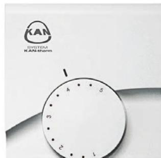
Basic heating/cooling electronic room thermostat is responsible for controlling executive elements - electric actuators in KAN-therm surface heating and allows for individual adjustment of temperature in a room. The thermostat can be mounted inside flush-mounted box or directly on a wall. It is available in 24V and 230V versions.
