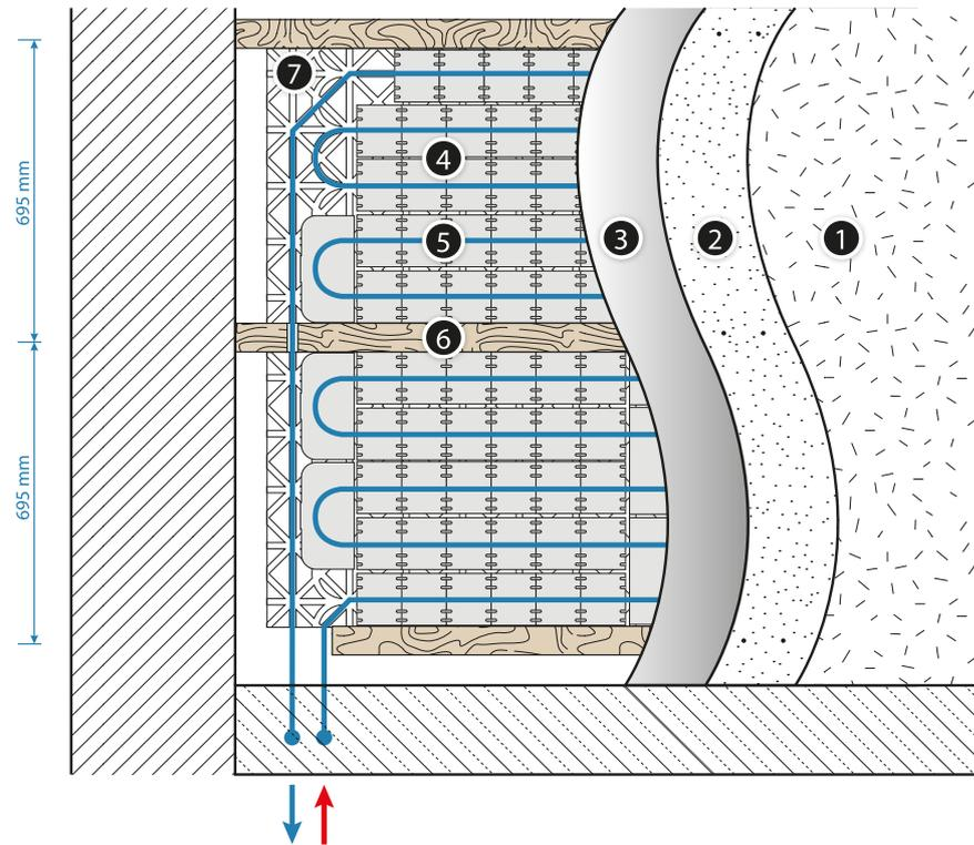
**Fig. 36.** KAN-therm TBS 14 board with steel radiating lamellae
