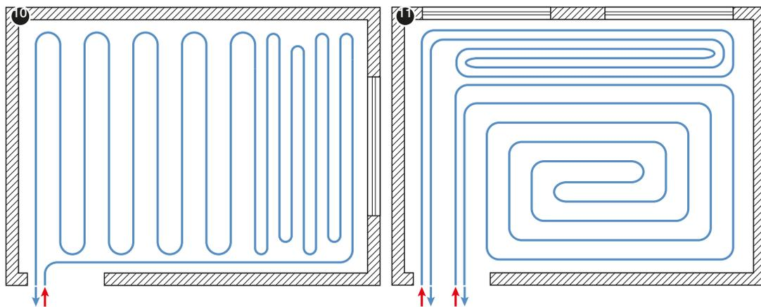
The heating loops should not be arranged under the room furnishing elements, which are built-in permanently (kitchen cabinets, bathtubs etc.).
