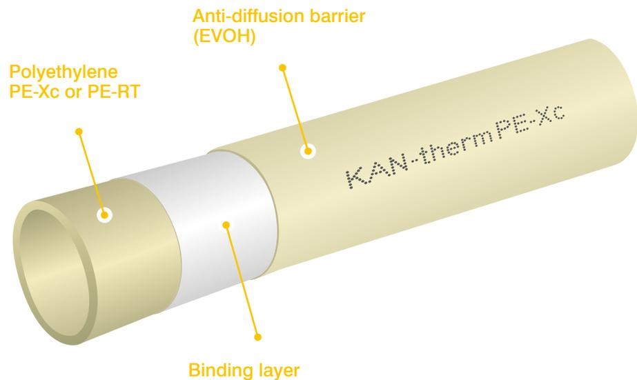
Fig. 48. Design of KAN-therm multilayer pipes
