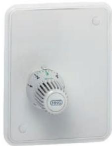
The device controlling temperature in a room regulates the flow of medium through single floor heating circuit, without additional heaters, depending on ambient temperature. Room set can be mounted both on the supply and return in floor heating circuit. Thermostat receives the ambient temperature and properly regulates the flow of water in a heating circuit.
