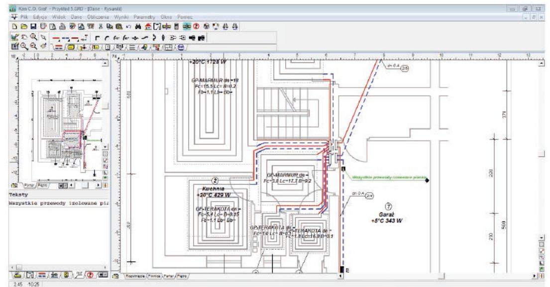
If the designer has floor plans drawn using software that generate WMF, DXF or DWG files (AutoCAD, CorelDRAW, MS Word, etc.), such files can be uploaded into KAN C.O. Graf. This gives heating installations' architect and designer an opportunity for close cooperation and contributes towards a significant reduction of the design process duration.
