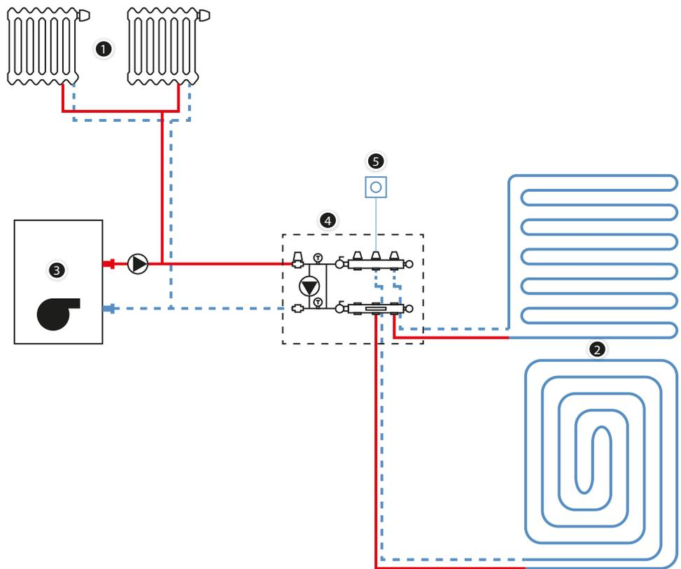
**Fig. 60.** Manifold provided with 77A (or 73A) mixing system
