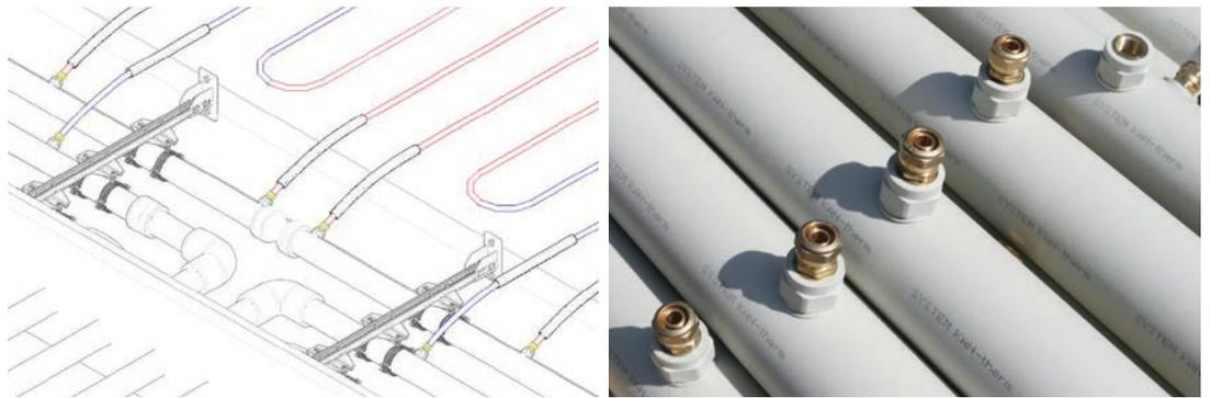
Possible configuration of KAN-therm PE-RT 18 × 2 mm heating pipes connection to KAN-therm PP Glass collector made of pipes of diameter 50 mm:
