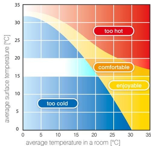
Surface heating/cooling systems are low temperature systems. Average temperature of heating/cooling surface is only slightly higher (or lower for cooling) than the air temperature within the space. For surface heating, temperature of 20°C provides the same thermal comfort as 21- 22°C achieved with traditional radiators on convection heaters.
