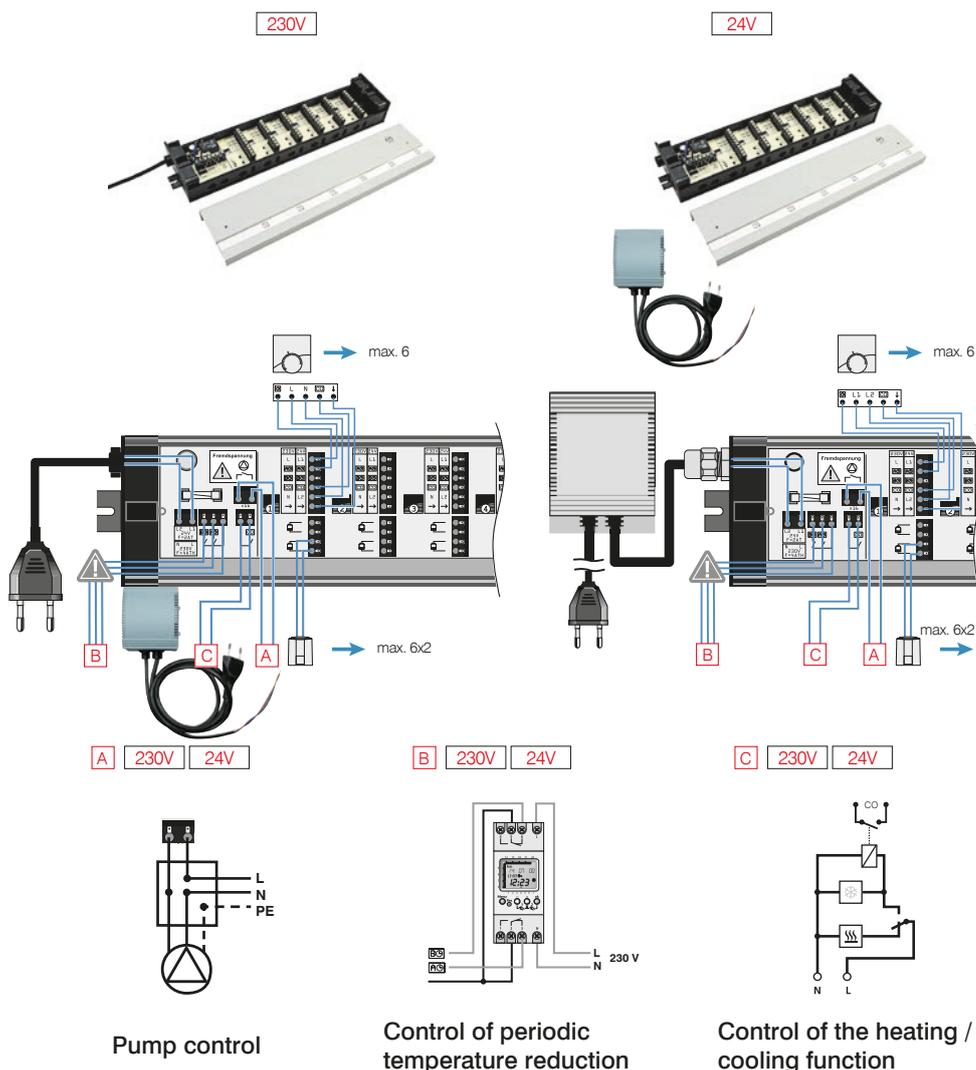
**!** Terminal block mounting and configuration in the “Basic 230/24V electrical terminal block for heating/cooling with a pump module” manual
