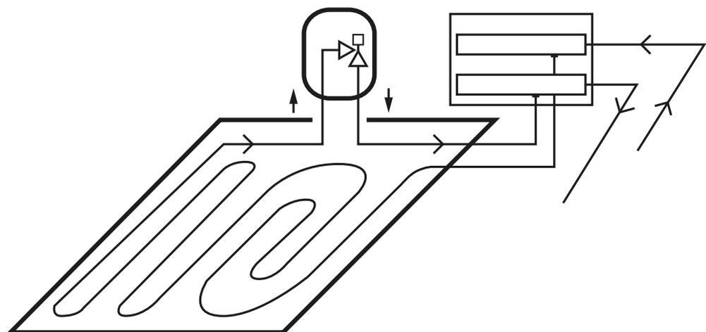
**i** “Surface heating unit with vent and thermostatic valve” Manual
