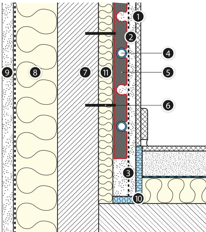
**Fig. 33.** KAN-therm heating pipes mounting in wall heating performed using wet method
