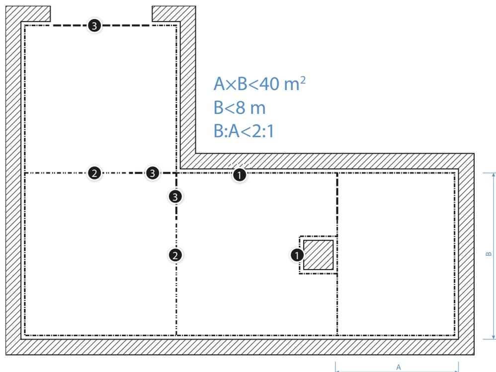
**Fig. 18.** Correct and incorrect distribution of heating field with a dilatation gap
