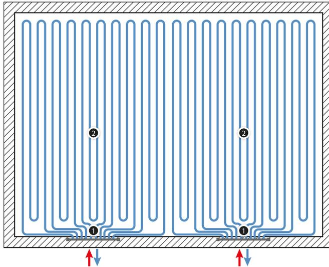
In the first case, the KAN-therm surface heating manifolds are used, which allow for a proper heat distribution and hydraulic adjustment of each circuit and heating section. Up to 12 heating circuits can be connected to a single manifold.
