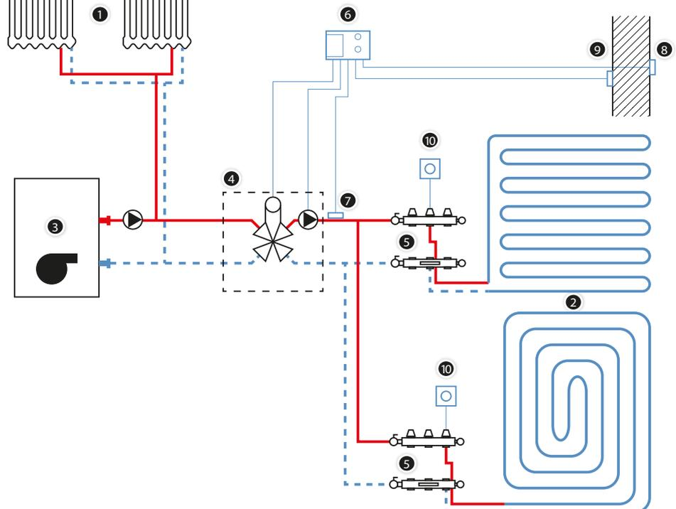
**Fig. 56.** Control elements of KAN-therm central mixing system (SM4 actuator (1) and weather regulator(2))
