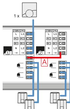
Fig. 70. Time control devices connection
