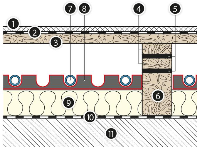
After the arrangement of thermal insulation, holes should be made in it, which shall be used for the accommodation of floor supports in accordance with the recommendations of sports floor supplier. The number of holes and spacing between them depends on the adopted type of a floor.
