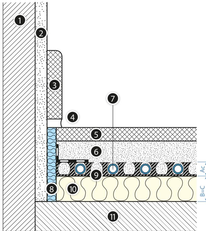
**Fig. 28.** Floor heater with KAN-therm Profil System board and supplementary insulation and damp-proof coating on the ceiling laid out on the ground
