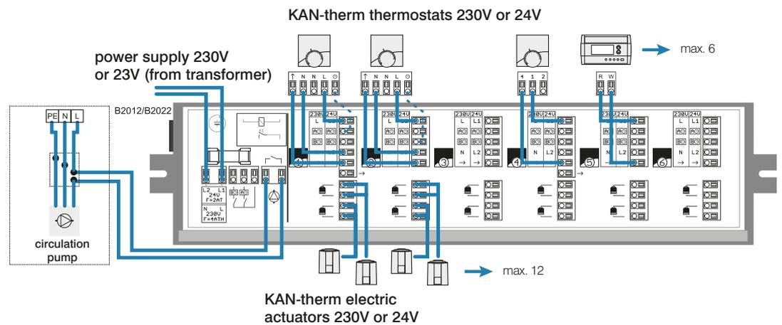
Normally one thermostat can control one or two actuators. If a jumper (A) is used, one thermostat can control 3 or 4 actuators.
