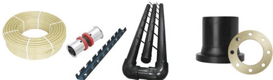
KAN-therm collectors are made of polyethylene pipes of diameter 160-180 mm with spigots of diameter corresponding to the heating loops pipes diameter and spacing, arising from the designed heating pipes spacing. Collector segments are connected by butt welding, it is also possible to connect them using electric resistance fittings. The collectors are performed and delivered in accordance with an individual technical documentation.
