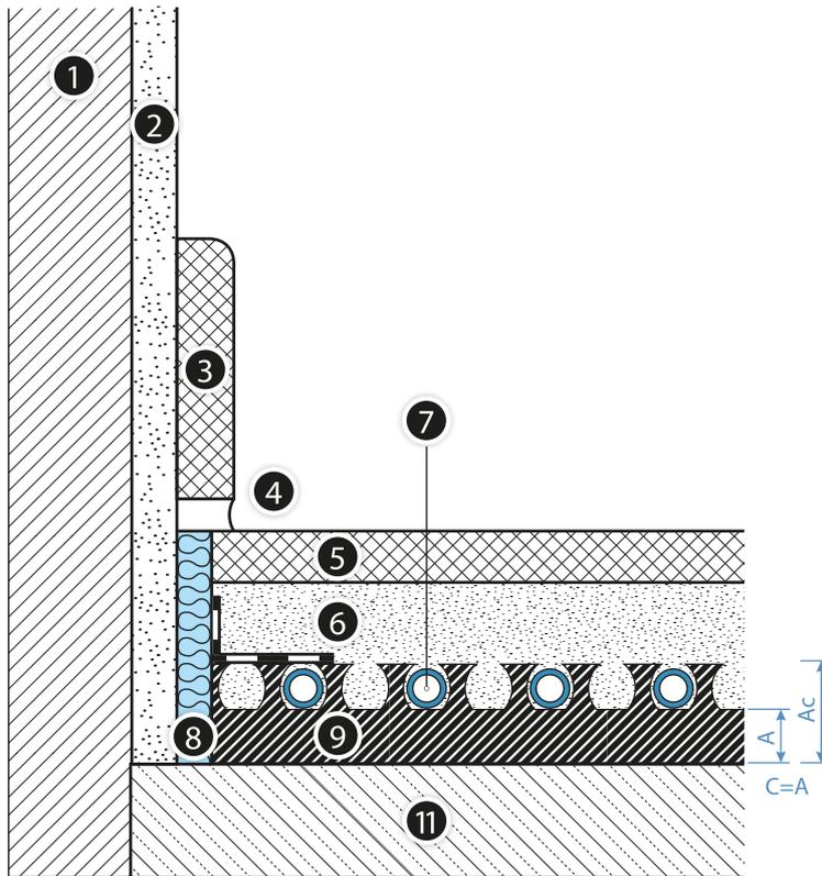
**Fig. 26.** Floor heater with KAN-therm Profil System board and supplementary insulation on the ceiling above internal not heated room and on the ceiling in contact with outside air
