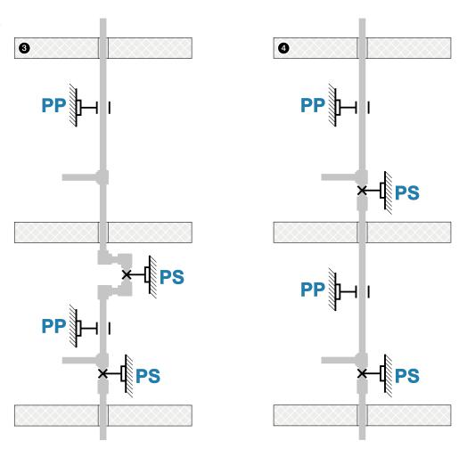
Maximum distances between supports for KAN-therm PP System uniform pipes depending on the diameter and medium temperature. For vertical pipeline sections, the distance between the supports can be increased byabout 30%.
